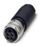
Connector, Universal, 4-position, Socket straight 7/8"-UNF, Screw connection, knurl material: Zinc die-cast, nickel-plated, cable gland Pg13,5, external cable diameter 10 mm ... 12 mm
