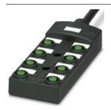
Sensor/actuator box, application: Standard, connection method: M12-SPEEDCON-socket Plastic, number of slots: 8, number of positions: 4, coding: A - standard, slot assignment: single, status display: yes, pnp; master cable connection: Fixed connection 180°, PUR/PVC, cable length: 10 m, shielding: no
