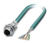
Assembled Ethernet cable, CAT6<sub>A</sub>, shielded, 4-pair, 26 AWG stranded (7-wire), RAL 5021 (water blue), M12 flush-type socket, rear/screw mounting with M16 thread to free cable end, length: 1 m
