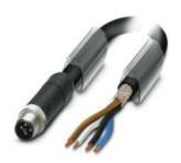
Power cable, 4-position, PUR halogen-free, black RAL 9005, shielded (Advanced Shielding Technology), Plug straight M12, T-coded, on free cable end, cable length: 10 m
