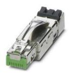
RJ45 connector, Degree of protection: IP20, Number of positions: 8, 1 Gbps, CAT5 (IEC 11801:2002), Material: Zinc die-cast, Connection method: IDC fast connection, Connection cross section: AWG 23-22, Cable exit: straight
