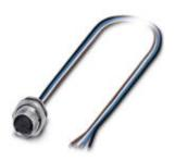
Sensor/actuator flush-type socket, 4-pos., M12 SPEEDCON, rear/screw mounting with M16 thread, with 0.5 m TPE litz wire, 4 x 0.34 mm²
