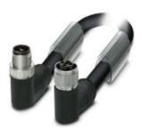
Power cable, 4-position, PUR halogen-free, black-gray RAL 7021, Plug angled M12, T-coded, on Socket angled M12, T-coded, cable length: 10 m
