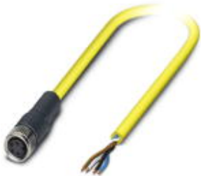
Sensor/Actuator cable, 4-position, PVC, yellow RAL 1021, free cable end, on Socket straight M8, Cable length: 2 m
