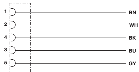
Contact assignment of the M12 socket
