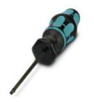
Torque screwdriver, with preset torque of 2.0 Nm and 4 mm hexagonal drive for the pressure nut of the fast connection
