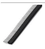
Taped ferrules, 1.5 mm², sleeve length 8 mm, with plastic collar, according to DIN 46228-4, black, for processing with the CRIMPFOX 4 IN 1, 10 strips each with 50 sleeves per strip.
