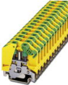
Protective conductor universal terminal block with bolt connection, cross section: 0.1 - 2.5 mm 2 , width: 9 mm, color: Green-yellow
