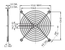
Welded, zinc-plated steel wire
