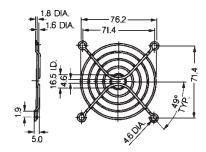
Welded, nickel chrome-plated steel wire
