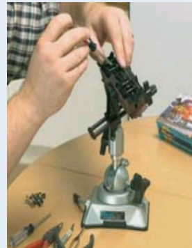
203 Head in a larger 380 Vacuum Base. An example of using PanaVise in a non-workshop setting.
