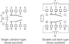
S : Coil polarity of set (operate) R : Coil polarity of reset (release)
