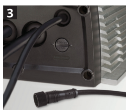
3 Waterproof Connector Port for Optional Charge Status Remote
