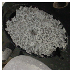
Unprotected and premature transom & outdrive zinc loss
