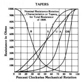
Tapers A, DB, S and U are measured between the wiper and the counter-clockwise terminals; taper B is measured between the wiper and the clockwise terminals.
