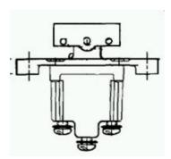
TP Series Rocker Switch, 1 pole, 3 position, Screw terminal, Above Panel Mounting
