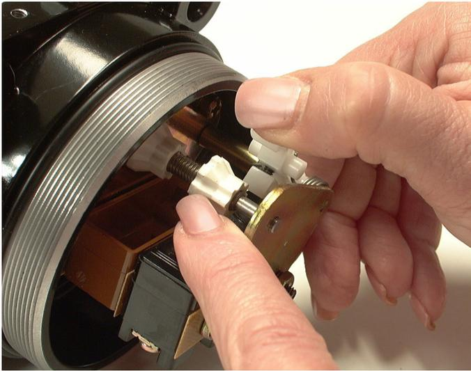
2. Turn cam wheel to be adjusted to desired position. Each notch on the wheel represents a change in operation point of 0,116 mm (.0045 in.). Moving the cam wheel in the direction away from the base housing advances the operate point. Pretravel **decreases** and overtravel thereby **increases**. When positioning cams, be sure the cam follower is allowed to utilize the full rise of the cam. This is required to provide adequate overtravel and release travel of the basic switches.
