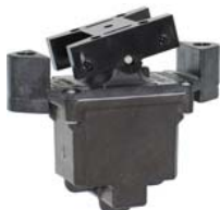
TP Series Rocker Switch, 2 pole, 2 position, IWTS (16-20 Gage) terminal, Above Panel Mounting
