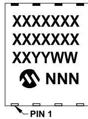
8-Lead DFN-S (6x5x0.9 mm)
