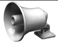
70-707-1  $8\Omega$  @ 10 watts 500Hz - 7.8KHz 5" diameter opening, 6" wire leads. White ABS plastic.
