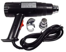
Voltage:120V/60HzAmperage:12AWatt:1440W2 fan speeds:Low & High2 heat settings:Approx. 850°F on Low, 1120°F on HighResetable thermostat protection
