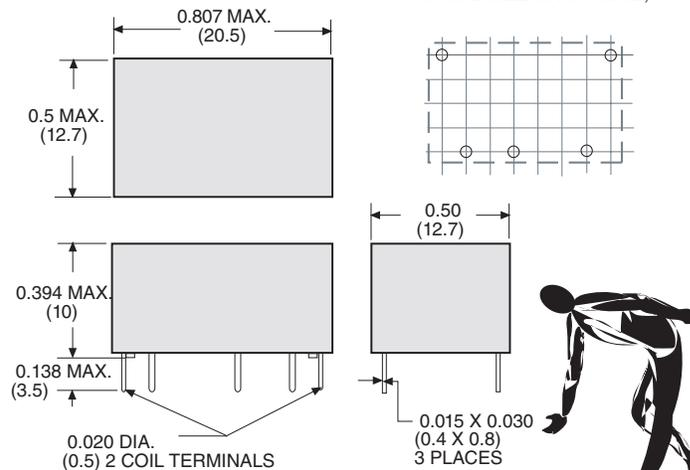
**PRINTED CIRCUIT MOUNTING HOLE LAYOUT**
