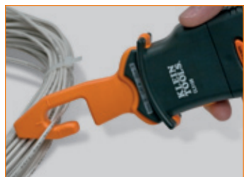
Separate Tie-wrapped Wires
