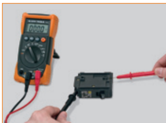
Measure Circuit Breakers
