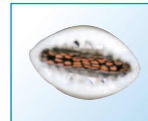
Diagonal cutters do not cut cleanly and decreases the quality of the strip.
