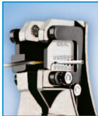
Die-type blades incorporate a counterbored hole sized to the insulation and an inner cutting hole sized to the conductor. This varies depending on insulation type and thickness.
