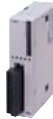
8-point Transistor Sink Output Module FC4A-T08K1 8 output points 0.3A transistor sink output Removable screw terminal
