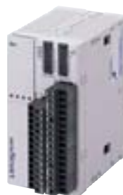
FC4A-D20RS1 12 input points 8 output points 0.3A transistor source output 24V DC 31.2KB memory 244 max I/O expandability 240V AC-2A/30V DC-2A relay output
