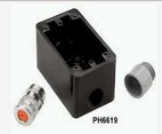
Black non-metallic FS box with 3/4" threaded hubs used for mounting phone and TV outlets and #PH6595 recreational vehicle inlet (see #PH6621 for mounting box on recreational vehicle). Cord connector included for strain relief and to maintain watertight integrity of box when cable is used. PVC adapter also included for connection of PVC conduit to box.
