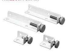
Provide additional support for panels on which heavy components are mounted. Each panel support fits over a collar stud and is then adjusted so the weight of the panel is partially supported by the bottom of the enclosure. Locknuts prevent accidental change in adjustment. A polyethylene-covered base on each panel support distributes the panel weight and prevents damage to the interior finish. Constructed of heavy-gauge steel. White finish.
