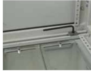
Secure bottom panel supports and upper panel mounting brackets into place. Upper panel mounting brackets feature a heavy duty collar stud. Notches in strut provide locating guidance.
