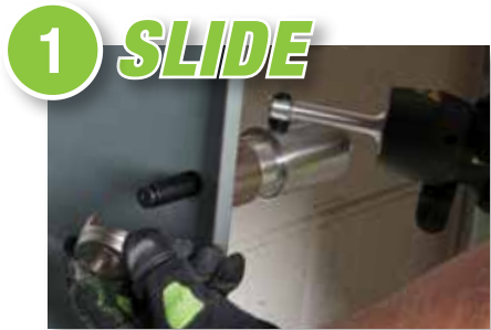
1 SLIDE Slide die and punch onto draw stud: “No-thread” design eliminates cross-threading.
