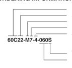
**Angle of Throw:** 22= 22.5° or 16 positions Rotation Torque: M= Medium torque
