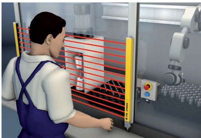
Finger, hand and arm protection on machines with the safety light curtain SLC
