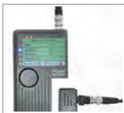
BNC coaxial cable test
