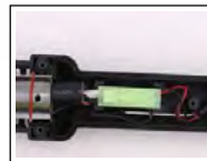
Connectorized design for quick change heater
