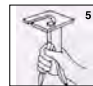
By turning the tool before each cut, a minimum radius can be cut.
