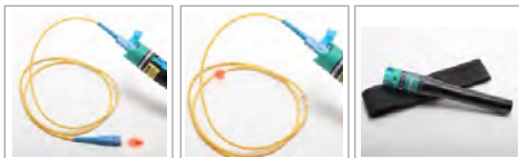
Continuity test Locate break point Accessory
