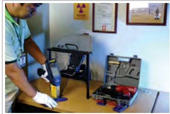
Handheld XRF for RoHS Compliance Testing
