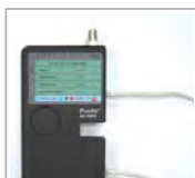
RJ11/12 telephone wire test
