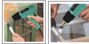
Paint and varnish removal
