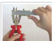
Outside diameter measurement
