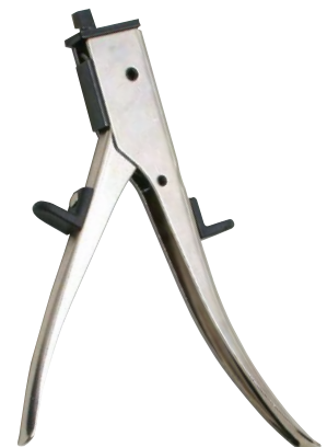
A scribe line can be followed by looking down on work in this position. A slot is cut by making successive cuts.
