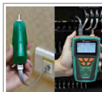
Verify LAN/ Telephone/ Coaxial cable condition
