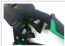
Stripping twisted pair round cable
