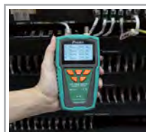
Locate break point and length measurement
