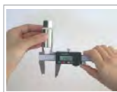
Inside diameter measurement
