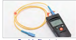
Break in fiber test
