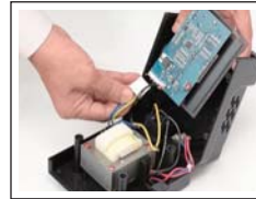
Modular design for easy repair(only for SS-207)
