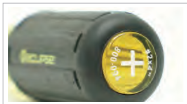
The screw symbol and tip size marking is on the handle end
