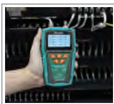
Locate break point and length measurement
