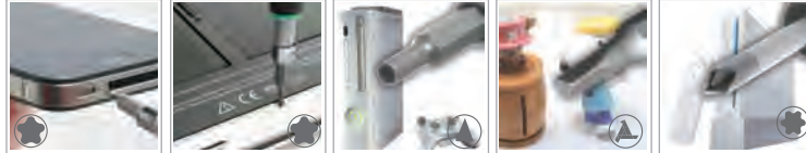
The P2/P5/P6 pentalobe tips are special for Apple products.
