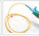
Locate break point
