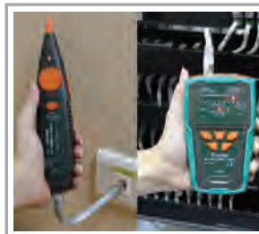
Verify LAN/telephone cable condition
