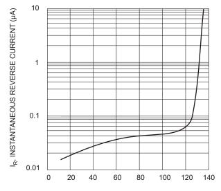
PERCENT OF PEAK REVERSE VOLTAGE (%) Fig. 5, Typical Reverse Characteristics
