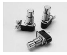
The 110/316-P-Series pushbutton switches are heavy duty, AC/DC rated and suitable as foot-switches. These switches are available with alternate or momentary action. This series is equipped with a quick-make, quick-break contact mechanism which is both nonteasable and self-cleaning. Typical actuation force ranges from 6-8 lbs.
