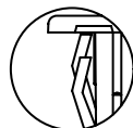
DETAIL VIEW VH1 HOLE PLUG (No wing serrations for ease of removal)
