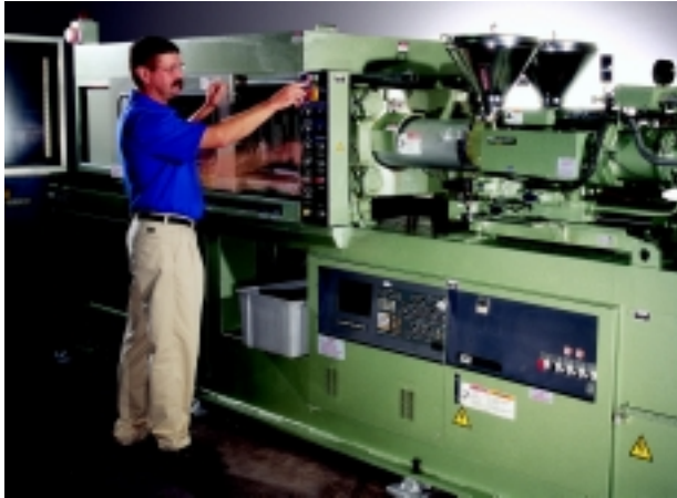
Two-shot injection molding of thermoplastic material
