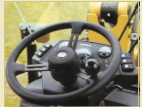
Operator control integrating rocker switches and custom controls
