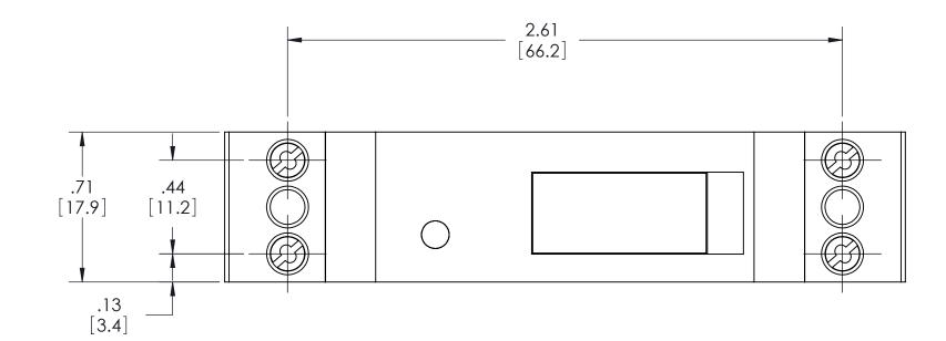
Tolerances: ± 0.02 in / 0.5 mm. All dimensions are in: inches [millimeters]
