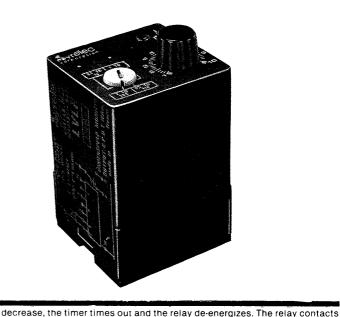
This straight forward underspeed detector can monitor all underspeed requirements (conveyors, worm reductions, pack-aging machines . . . etc.) where it is essential that loss of speed or stopping gives an alarm. The input information sensor for the speed can be a proximity switch, voltage level or contact closure.
