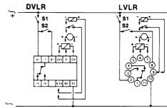
The external contact S2 for reset and inhibit should be isolated from all other circuit (12V, 3 mA)
