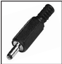
30-336 Coaxial AC/DC power plug. 1.0mm I.D. 3.8mm O.D. .17" cable opening.
