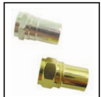
75-534-PL Nickel 75-534G-PL Gold Plenum RG6 "F" Connectors. Plenum connectors in gold or nickel. Threaded interior crimp for secure cable installation. Connector face has waterproof boot to prevent moisture from contaminating the connection.
