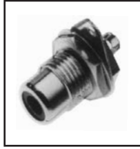
30-424-Co Lo R RCA Audio Jack. Locking nut fits on front of panel. Shallow mounting depth. Mounts in 3/8" hole. Bushing length .26" Available with black, red, white and yellow inserts. Please specify color when ordering
