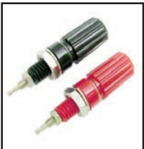
90-799 Black 90-800 Red 5-way binding posts. Plastic insulation. Has .1875" keyed threaded mounting shaft. Mounts in panels up to .25" thick.
