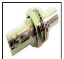
75-521 Panel feed thru connector. BNC Female to RCA Female. Bushing dia.: .487" Bushing length: .33" Overall length is 1.29" Mounts in .5" hole. 75 ohm. 75-521-50 50 Ohm version
