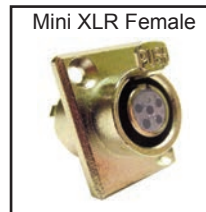
30-643-3 3 pin 30-643-4 4 pin 30-643-5 5 pin 30-643-6 6 pin Chassis mount MINI Female XLR. Mounts in 15.20mm, .60 hole. Nickel plated body.
