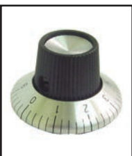
85-567 Chrome-skirted instrument knob. Calibrated 0-9. Fluted ebony grip with aluminum insert for \frac{1}{4} -inch shaft with set screw. (Diameter \frac{3}{16} " ) .68" high.
