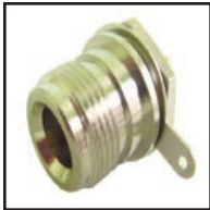
75-572 Chassis mount Female "N" connector. Over all length is 1.09\". Mounts in chassis .62\" hole.
