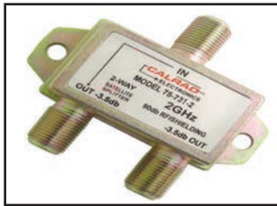
75-731-2, 2-Wa Y 2GHz, 90dB Sat ELLIt E SPLIt t Er Power passive to all ports. Insertion loss 4-4.5dB max. Port-Port isolation 12-15dB min. Input return loss 12-15dB min. Zinc alloy die cast housing.
