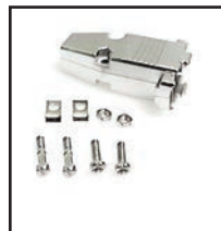
30-553m (Nickel) 30-553m-g (Gold) DB9, DB15HD metal housing for 10-11mm cable, with hardware. 2-piece construction, for use with DB9, DB15 type connectors.
