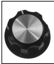
85-574 Black bakelite, aluminum insert. Fluted grip, \frac{1}{4} -inch brass bushing with set screw. 1 \frac{5}{16} " Diameter, \frac{5}{8} " high.
