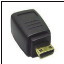
35-706 HDMI Female to mini HDMI Male adapter. Gold plated contacts.
