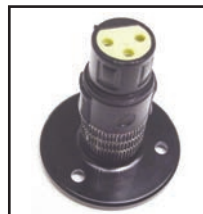
30-590 Chrome 30-590-Bk Black Female XLR desktop mount in, used for quick release style gooseneck mics. Removable solder type Female XLR. Mounts with 3 screws included. Base dia. 1.75", height 2".
