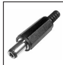
30-375 DC coax power plug. 3mm I.D., 6.3mm O.D., 9.5mm long. With strain relief. .20" cable opening.
