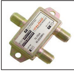
75-705-a Sat ELLIt E DIPLEXEr -MIXEr Size: 2.25" X 2" X 5/8" (W/D/H) 5-2050MHz satellite splitter-combiner separates or combines off-air TV antenna and satellite signals from a single feed-line. High performance printed board circuitry. Anti-Corrosion chromate zinc-alloy die cast housing 90dB min RFI shielding - epoxy sealed back cover. .5" precision machined 'F' connector threads. DC pass-through current 500mA max. Insertion loss VHF-UHF 0.5dB - satellite 1.5dB. Isolation VHF 25dB - UHF 20dB - satellite 23dB. Return loss VHF 18dB - UHF 10dB - satellite 12dB.
