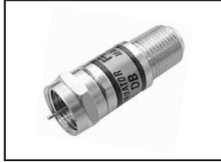
75 Ohm INLINE attENUatOr 0-1750MHz. Female to Male "F" attenuator. 5% tolerance with return loss of 20dB. 22 gauge spring steel center. DC power blocking. 75-720-3 ..... 3dB attenuation 75-720-6 ..... 6dB attenuation 75-720-8 ..... 8dB attenuation 75-720-10 ..... 10dB attenuation 75-720-16 ..... 16dB attenuation 75-720-20 ..... 20dB attenuation
