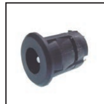
30-720-2.1 2.1mm version 30-720-2.5 2.5mm version Chassis mount snap-in coax power jack. Nickel plated connector with black molded trim. Mounts in .375" hole, up to .07" panel thickness
