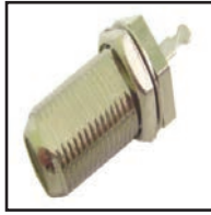
75-604 Chassis mount "F" Female connector. Mounts from rear with hardware. Mounts in .375" chassis hole.
