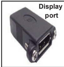
35-729 Display port panel mount feed-thru female to female jack. Mounts in a standard DB9 cutout. Gold plated contacts, includes mounting hardware.
