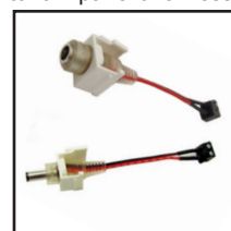
30-730 2.1mm solderless inline DC Coax power plug. 30-731 2.1mm solderless inline DC Coax power jack.
