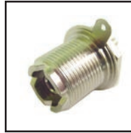
30-468 S0-239 Coax chassis connector (bullet-type). 5/8" hole size.
