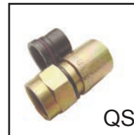
75-533-SN59 RG-59 75-534-QS Quad RG-6 "F" snap-n-seal connector is environmentally sealed to protect drops from harsh environments. Through a unique 360° compression process, this type of connector provides protection against signal leakage, required for today's high-bandwidth CATV systems. Use with Calrad 75-599A or 75-598 compression tool.
