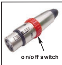
30-638 3-Pin XLR inline Female with labeled on/off switch. Shorts pins 2 & 3 to mute signal voltage with plastic noiseless switch. Gold plated contacts.
