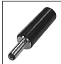
30-372 Coax power plug. 1.3mm I.D. 3.5mm O.D. 9.5mm long. .15" cable opening. 30-372-p With strain relief. .16" cable opening.
