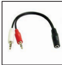
35-475 Two 3.5 mm stereo plugs to one 3.5 mm stereo jack, shielded. 10" long.
