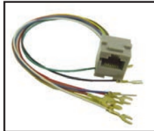
70-511 Modular Female chassis jack. 8-position, 8 wires and lugs. For 8 conductor cable equipment.
