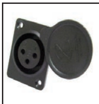
30-517 Isolated plastic Female XLR with protective cover. 3-pin Female XLR mounts in 15/16 " hole and requires a special cut out in order to mount.
