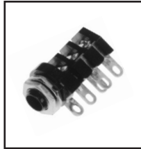
30-398 1/4" Audio Jack. 3-Circuit, 2 Closed. 3/8" bushing, Mounts in .355" hole.
