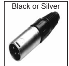
30-529-Bk 30-529-sL XLR 3-pin Male plug, twist-on strain relief. .15" to .3" cable opening. Internal compression style cable strain relief.
