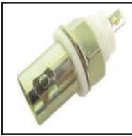
75-514 BNC Female, isolated ground from chassis. Length is 1.06". Mounts in .37" chassis hole. Bushing length .38".
