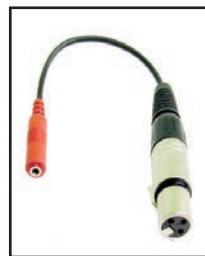
35-467 3.5mm stereo Female jack to XLR Female plug. Wired: pin 1 = ground pin 2 = tip pin 3 = ring. 8" long with Black PVC jacket.
