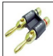
30-604-Bk Black 30-604-RD Red Dual gold banana plugs. For up to 8 gauge wire. .15" cable opening. 0.75" centers.
