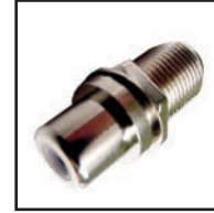
75-635G Gold Female to RCA to "F" bulkhead connector. Panel mount double "D" connector mounts in 3/8" hole. Overall length .95". "F" thread length .57". Mounting hardware included.
