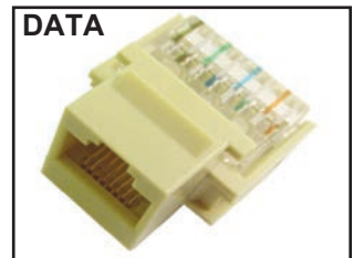
DATA 8-POSITION UL KEYSTONE MODULAR JACK IDC type meets level 3 & 4 requirements. 30 microns gold plated contacts and ABS material UL94/A-O. Suitable for 22-26 AWG wire. 72-101-BK ..... Black 72-101-IV ..... Ivory 72-101-WH ..... White
