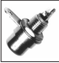
30-428-Co Lo R Nickel Gold 30-428g -Co Lo R Gold Nickel plated RCA Audio Jack with hex nut and solder lug. Single hole mount. 1/4" hole. Bushing length .25" Available with black, blue, green, orange, red, white and yellow inserts.
