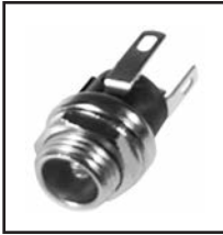
30-310 2.1mm 30-311 2.5mm. Chassis mount coax power jack. Insulated housing mounts in \frac{5}{16} " hole. N/C switch. 5.5mm O.D.
