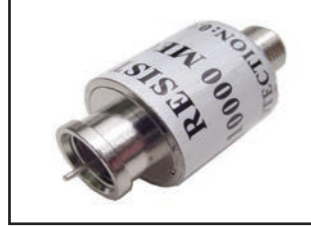
75-479 COaXial SUR GE and SPIKE Pr Ot Ect Or Protects cable, TV converters, decoders, satellite receivers, access cards, VCRs and TVs from incoming surges and electrical spikes. Uses a standard Male-Female "F" connectors. Frequency: 2GHz. DC passive, Impedance: 75 Ohms, Insertion loss: .2dB.
