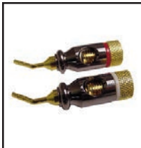
30-609-RD Red 30-609-Wh White Speaker terminals with solder/solderless speaker pin. White or red color band. Accepts 8-18 awg. cable. Gold plated with black chrome finish.
