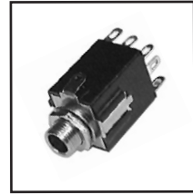
30-385 Stereo 1/4" Audio Jack. with DPDT normally closed and normally open circuits.
