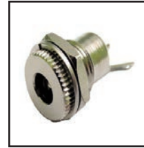
30-378 Japan 30-378-t Taiwan 2.5mm I.D. 5.5mm O.D. chassis mount coax power jack. For \frac{7}{16} " dia. hole in panels up to \frac{3}{16} " thick.
