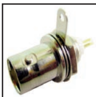
75-543 BNC Female chassis connector. Overall length is 1.08". Mounts in .375" chassis hole. Bushing length .28". 75-543G Gold version. 75-697 75 ohm version.
