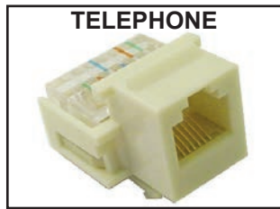
TELEPHONE 6-POSITION UL KEYSTONE MODULAR JACK IDC type meets level 3 & 4 requirements. 30 microns gold plated contacts and ABS material UL94/A-O. Suitable for 22-26 AWG wire. Will work as a 4 position jack. 72-100-AL ..... Almond 72-100-BK ..... Black 72-100-IV ..... Ivory 72-100-WH ..... White
