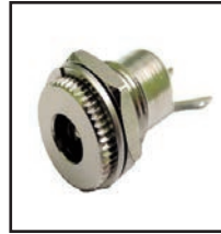
30-377 Japan 30-377-t Taiwan 2.1mm I.D. 5.5mm O.D. chassis mount coax power jack. Mounts \frac{7}{16} " dia. hole in panels up to \frac{3}{16} " thick.
