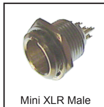
30-642-3 3 pin 30-642-4 4 pin 30-642-5 5 pin 30-642-6 6 pin Chassis mount MINI XLR Male. Mounts in .43" "D" hole. Nickel plated body.
