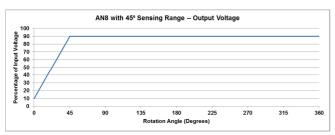
These charts show the output voltage as a percentage of the input voltage for a given angle of rotation. Example: 180<sup>o</sup> sensing range, magnet rotated 135<sup>o</sup>, output voltage will be 70% of input voltage (see dashed lines in graph above).
