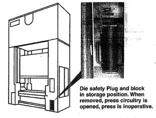
The receptacle is wired in-line with the machine control circuitry. The shorting plug is secured to safety equipment by a short length of chain. When the internally jumpered plug is engaged, it completes the circuit permitting the equipment to function.
