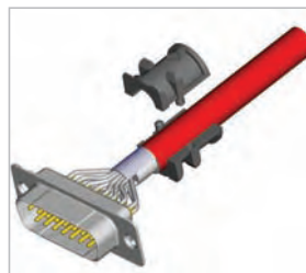
Attach the strain relief around the cable
