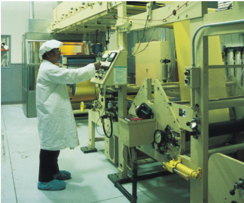
At Bergquist's Cannon Falls, MN, manufacturing facility, a Sil-Pad material runs through a 3-story coating press.
