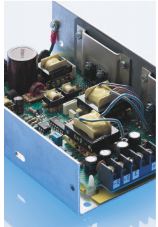
The application above uses punched parts to insulate the transistors from the mounting bracket and a sheet of Sil-Pad to isolate the mounting brackets from the frame of the assembly.
