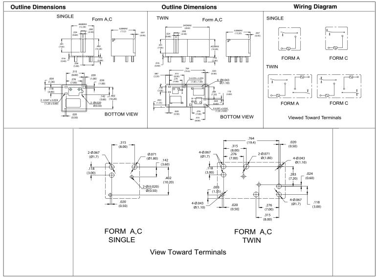
Dimensions in inches with millimeters in brackets below. Tolerance: ± .010"
