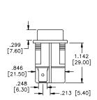
Double pole - quick connect terminals - curved actuator
