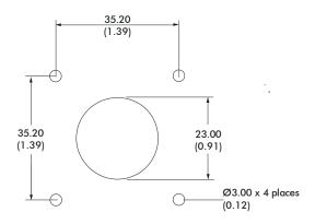
The body of the joystick is mounted from beneath the panel. The boot is passed through the panel cut-out and is held onto the front face of the panel by the mounting bezel. The square bezel has a gloss finish and is designed for use with No.4 x 3/8'' pan head self tapping screws whereas the circular bezel has a matt finish and is designed for countersunk screws.
