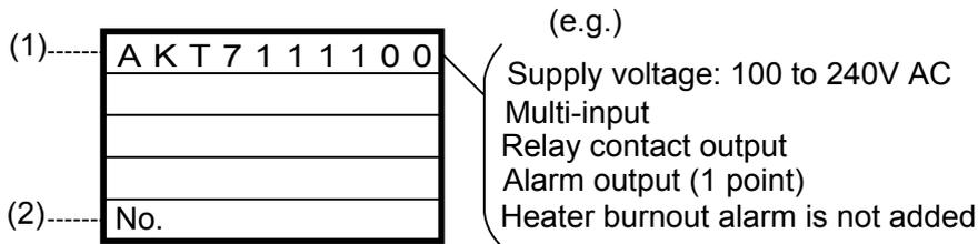
(1) Model number, supply voltage, input type, output type, etc. are entered.
